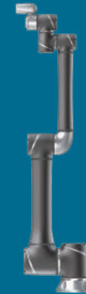
TM12M : Applicable for mobile stacking and mobile Machine Tending.
